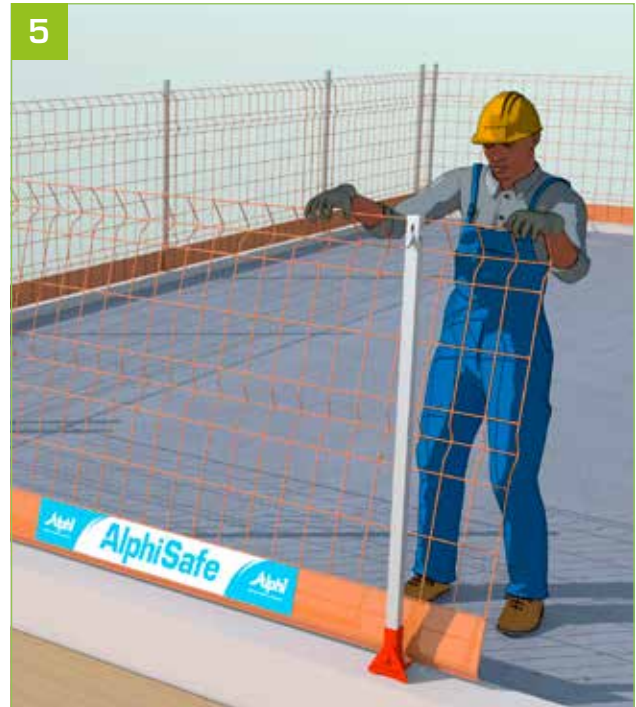
- Install the mesh, making sure that the baseboard is engaged in the adapter notch and the top in the opening provided.
