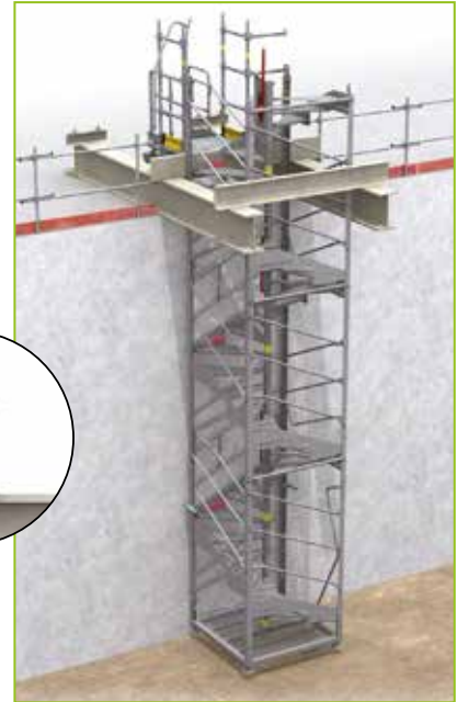
- Diagram of suspended Escalib MDS for groundworks floor access.
