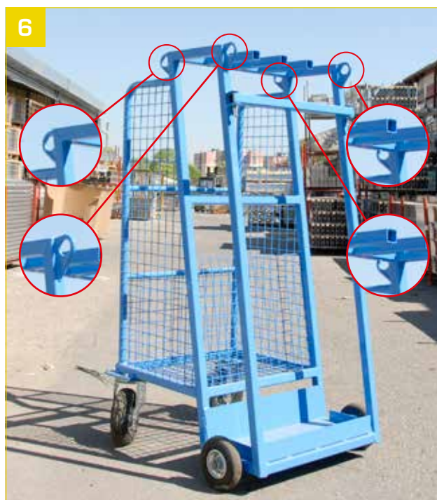
- Slinging: 4 hooks are used to handle the trolley, with props, using the crane.
