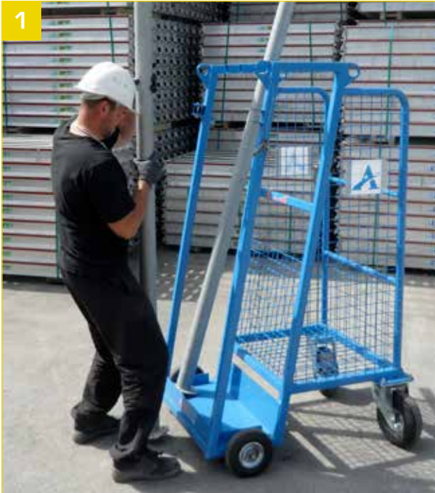
- Arrangement of props in vertical position.
