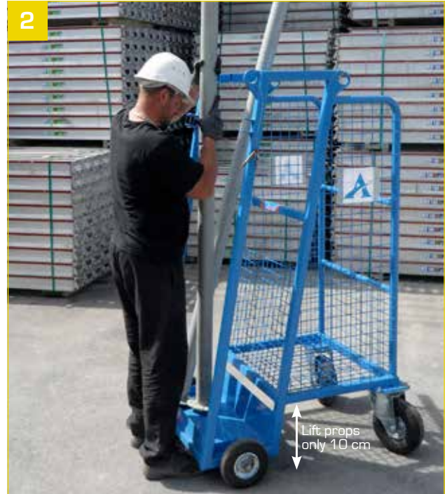
- Placing props in the trolley.
