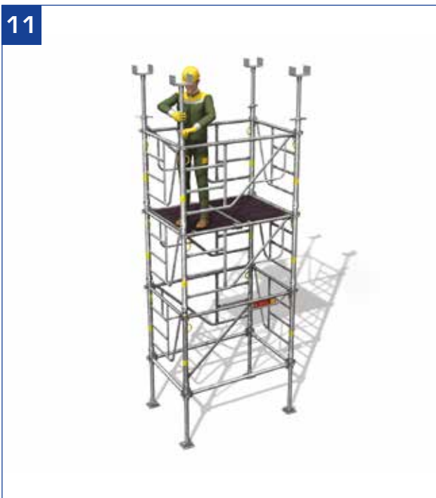
- Set up and adjust the head jacks.
