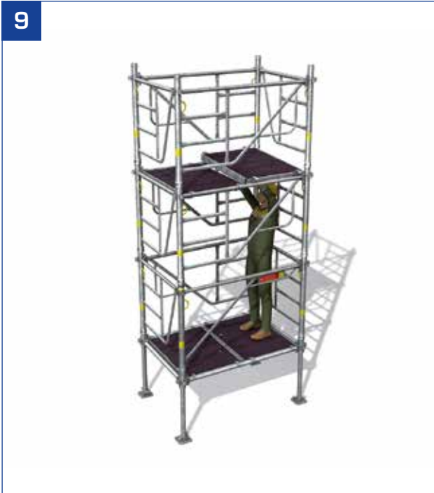
- Move the 2 nd plank with trapdoor from the lower level.
