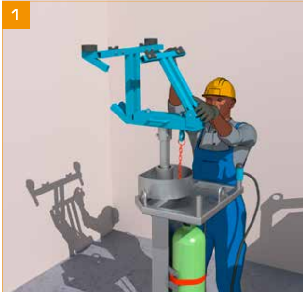
1 - Open out the rear arm of the MaxUp and lock it.
