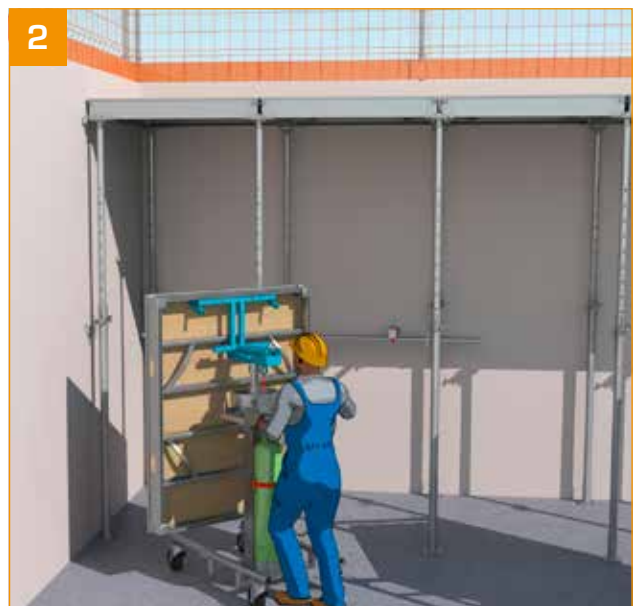
- Move the MaxUp to continue the formwork phase.
