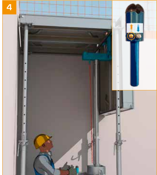
- Raise the panel to the desired height: the top edge must be aligned with the top of the panel already in place.
